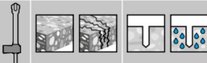
d<sub>0</sub>: 10 ... 35 MM | h<sub>ef</sub>: 60 ... 1000 MM
